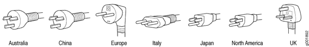
Figure 9: AC Plug Types
