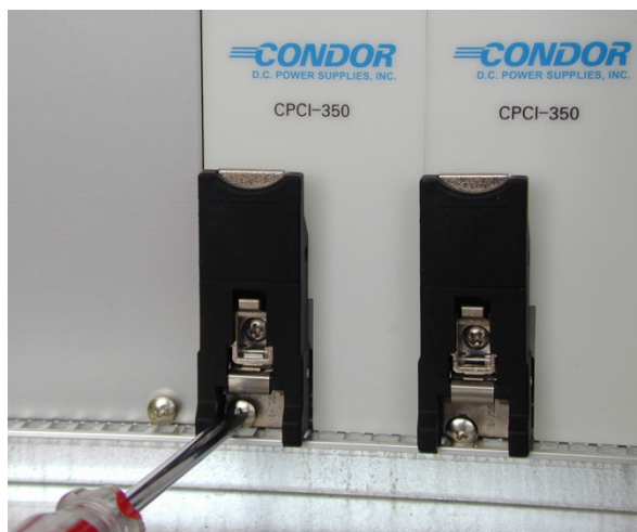
Figure 2-12 Removing a Power Supply
