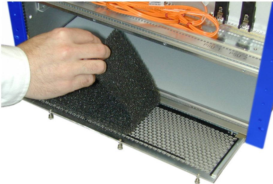
Figure 2-17 Removing the Air Filter
