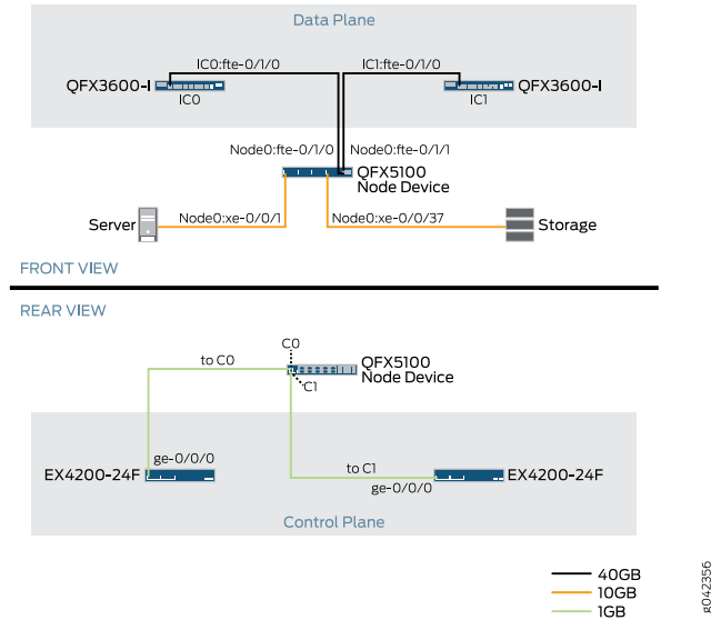
Figure 85: QFX5100 Node Device Data Plane Connects for QFX3000-M QFabric System
