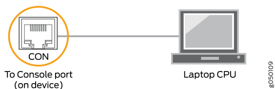
Figure 37: Connecting the QFX Series Directly to a Management Console
