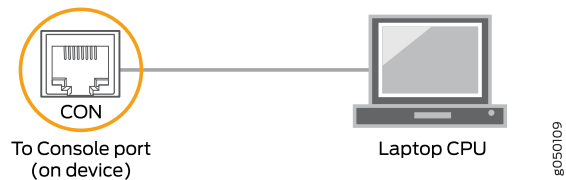
Figure 62: Connecting the QFX Series Directly to a Management Console
