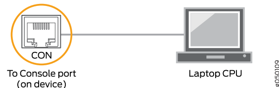
Figure 27: Connecting the QFX Series Directly to a Management Console
