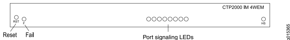
Figure 1: CTP2000 4W&EM Module
