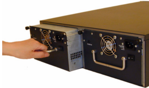
Figure 27: Removing an AC Power Supply
