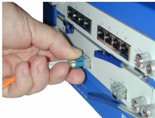
Figure 23: Ejecting the Cable
