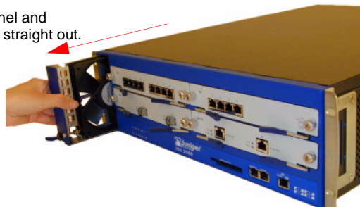
Figure 35: Removing the Fan Tray
