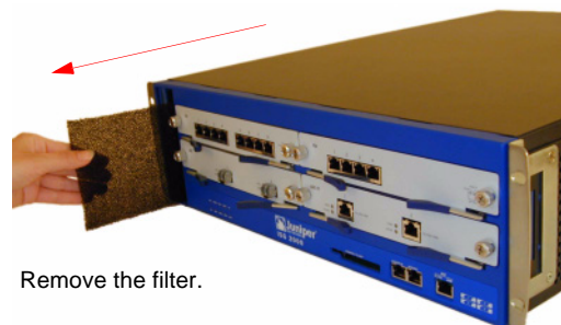
Figure 37: Removing the Fan Tray Filter
