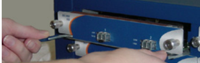
Figure 13: Interface Removal
