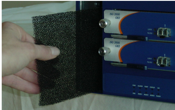
Figure 22: Removing the Fan-Tray Filter
