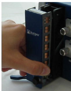
Figure 20: Removing the Fan
