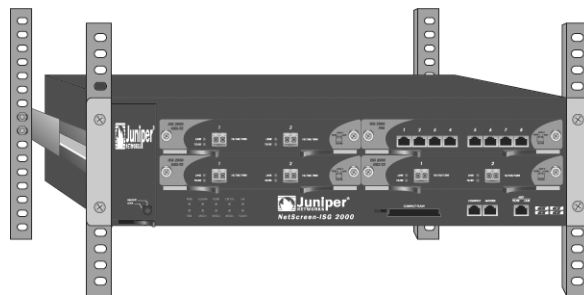
Figure 7: Front-Rear Mount for ISG 2000
