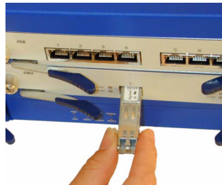
Figure 27: Installing the Transceiver
