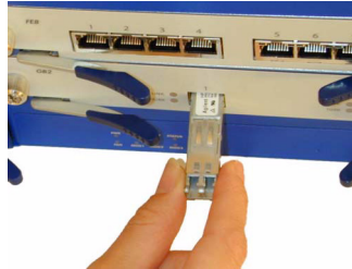
Figure 23: Sliding the Connector into the Transceiver Port
