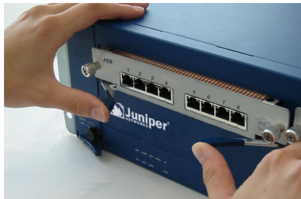
Figure 13: Lock Interface Module
