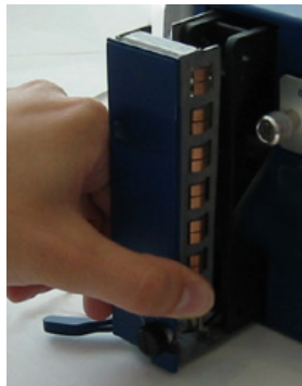
Figure 14: Removing the Fan
