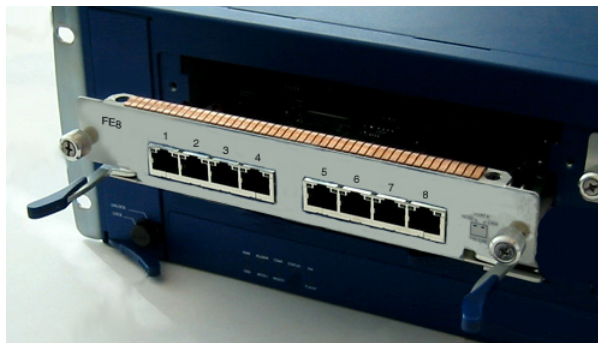
Figure 12: Insert Interface Module
