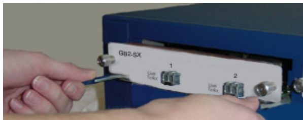
Figure 11: Remove Interface Module
