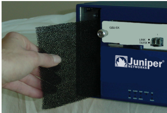
Figure 16: Removing the Fan-Tray Filter
