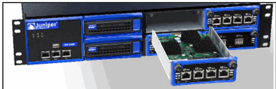
Figure 23: Replacing a Blank Tray with an I/O Module Tray
