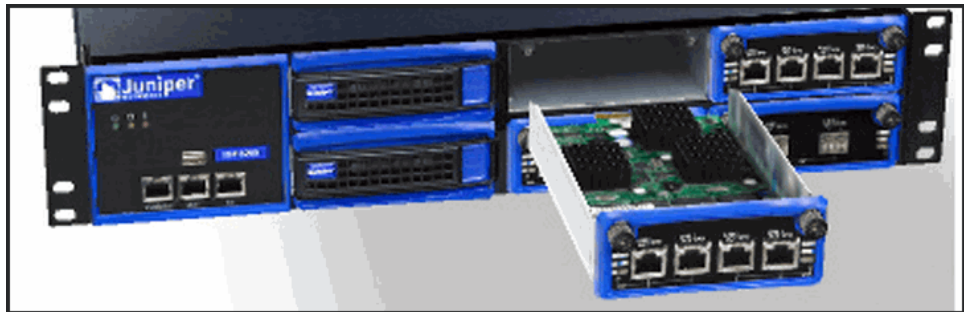
Figure 138: Replacing a Blank Tray with an I/O Module Tray
