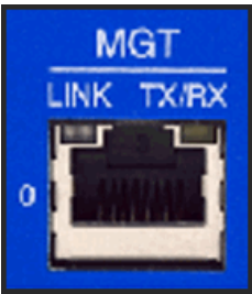
Figure 2: Management Interface Port LEDs
