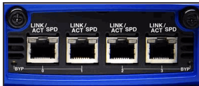
Figure 3: Copper Port LEDs
