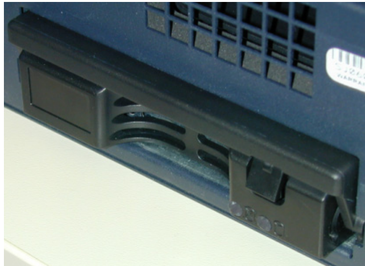
Figure 27: Hard Drive Latch in Closed Position
