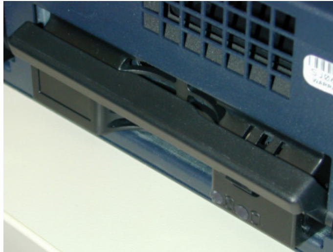
Figure 23: Hard Drive Latch in Open Position, Handle Released
