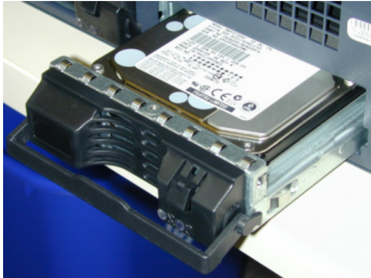
Figure 26: Drive Partially Inserted
