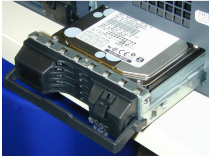
Figure 25: Drive Partially Removed
