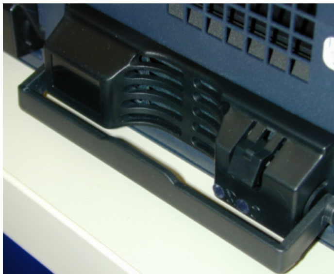
Figure 24: Hard Drive Handle Down
