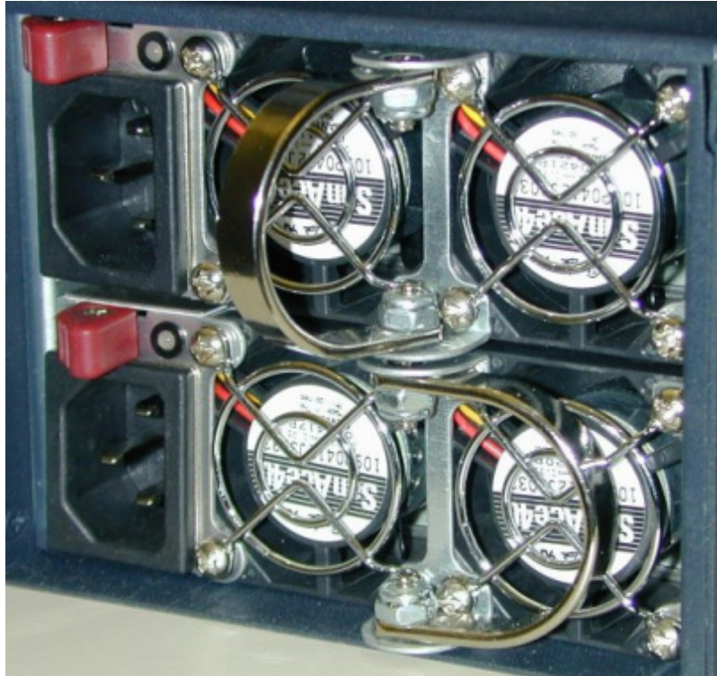
Figure 21: Power Supply Handles in Open and Closed Positions
