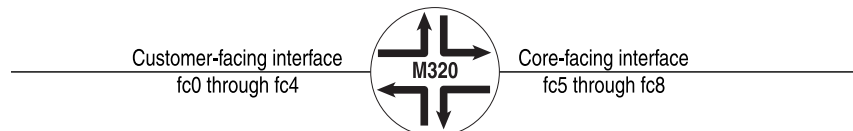
Figure 7: Customer-Facing and Core-Facing Forwarding Classes
