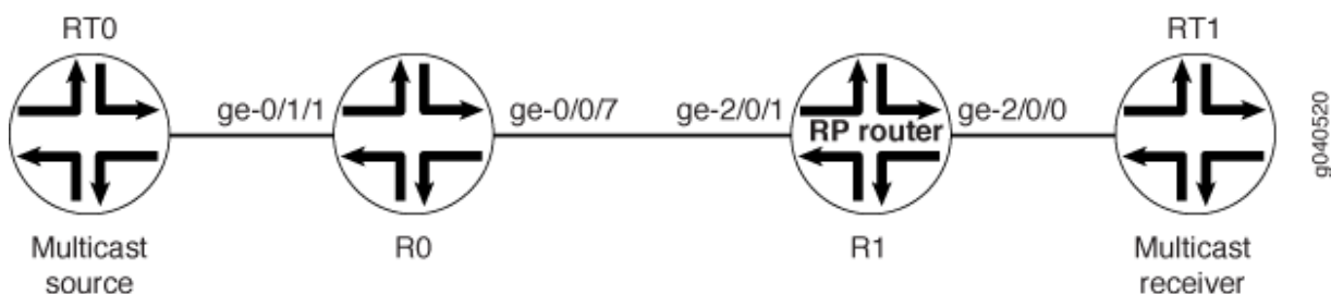
Figure 45: PIM Sparse Mode over an IPsec VPN
