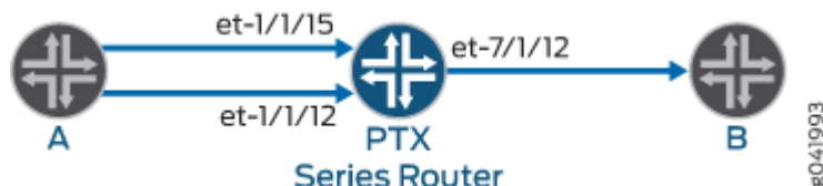
Figure 62: Topology for Configuring Strict-Priority Scheduling on a PTX Series Router
