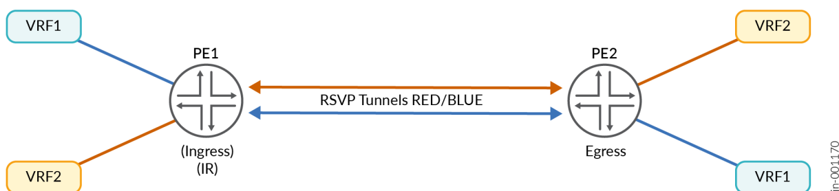
Figure 58: Selecting provider tunnels during Ingress Replication
