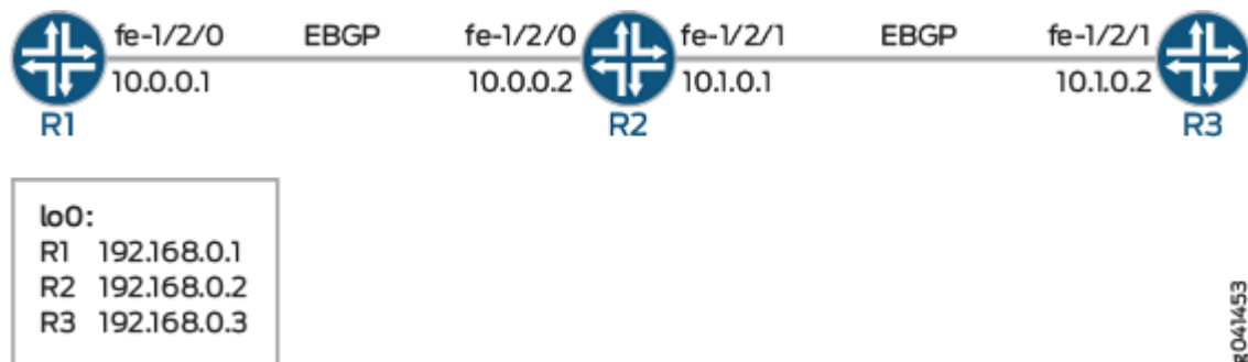
Figure 36: BGP Flap Damping Topology
