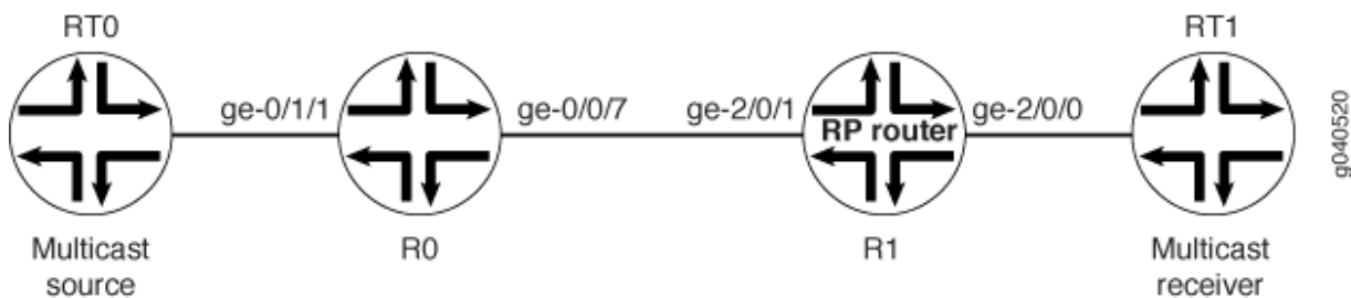
Figure 45: PIM Sparse Mode over an IPsec VPN
