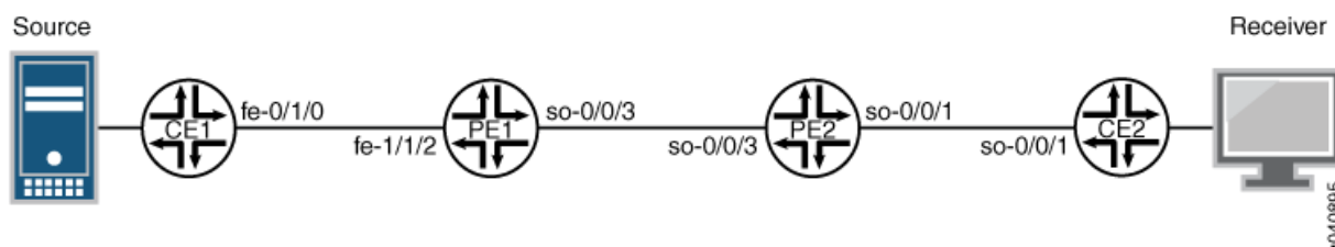
Figure 87: Different Provider Tunnels for IPv4 Multicast VPN Traffic
