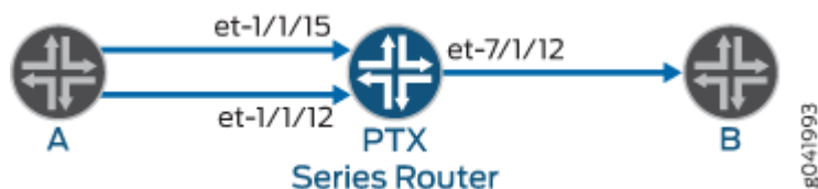
Figure 62: Topology for Configuring Strict-Priority Scheduling on a PTX Series Router
