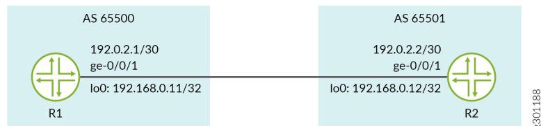
Figure 4: Topology for BGP Authentication
