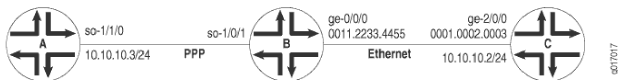
Figure 131: Sample Topology of Layer 2.5 Translational Cross-Connect
