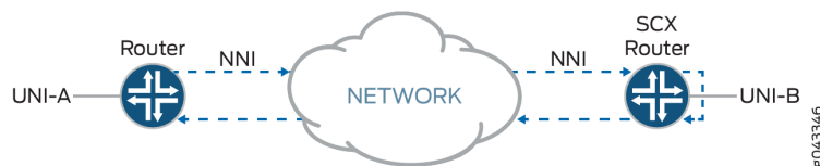
Figure 72: Testing End-to-End Service in Ethernet Loopback Mode
