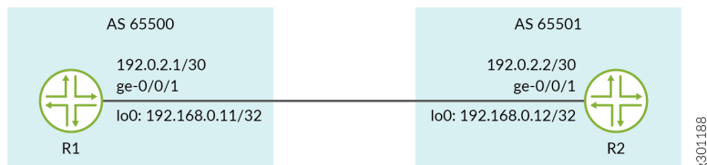
Figure 4: Topology for BGP Authentication
