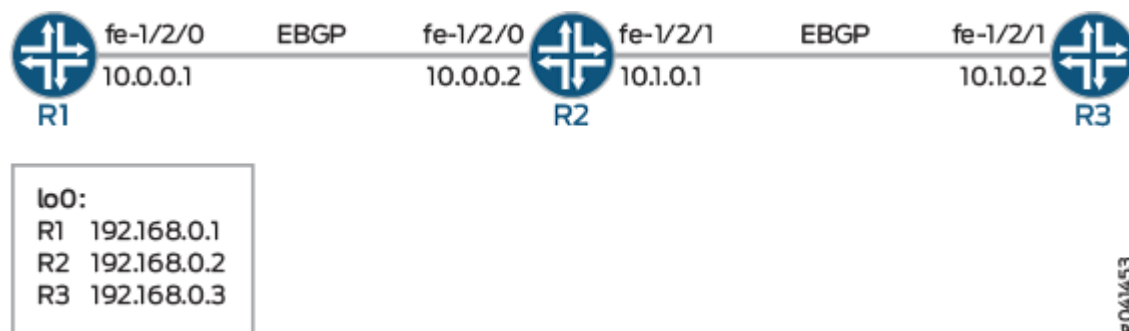
Figure 36: BGP Flap Damping Topology
