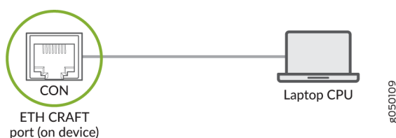
Figure 52: Connecting the QFX Series Directly to a Management Console
