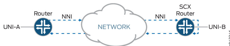
Figure 72: Testing End-to-End Service in Ethernet Loopback Mode
