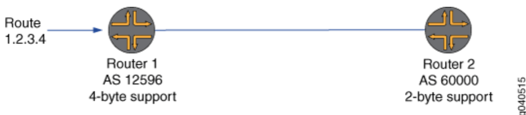
Figure 26: 4-Byte Capable Router Having a Peer Relationship with a 2-Byte Capable Router Using a 2-Byte AS Number
