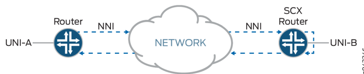
Figure 69: Testing End-to-End Service in Ethernet Loopback Mode
