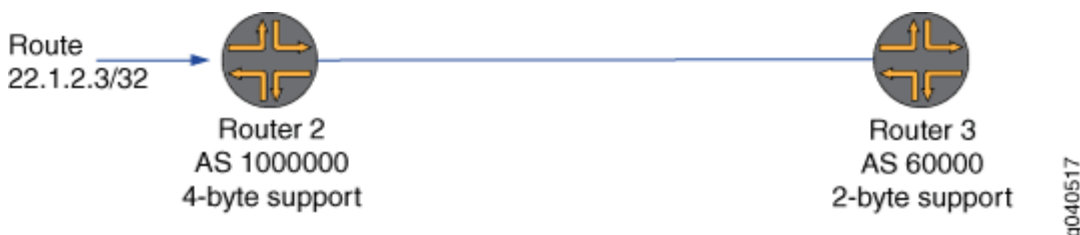
Figure 27: 4-Byte Capable Router Having a Peer Relationship with a 2-Byte Capable Router Using a 4-Byte AS Number
