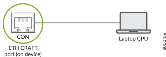
Figure 74: Connecting the QFX Series Directly to a Management Console
