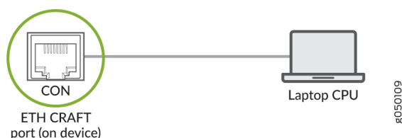
Figure 23: Connecting the QFX Series Directly to a Management Console
