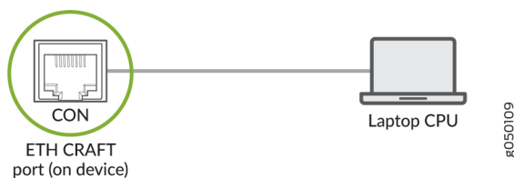
Figure 53: Connecting the QFX Series Directly to a Management Console
