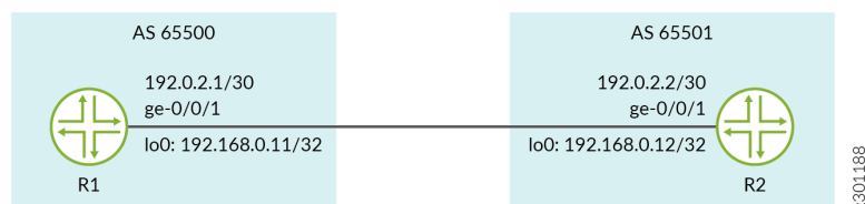
Figure 4: Topology for BGP Authentication
