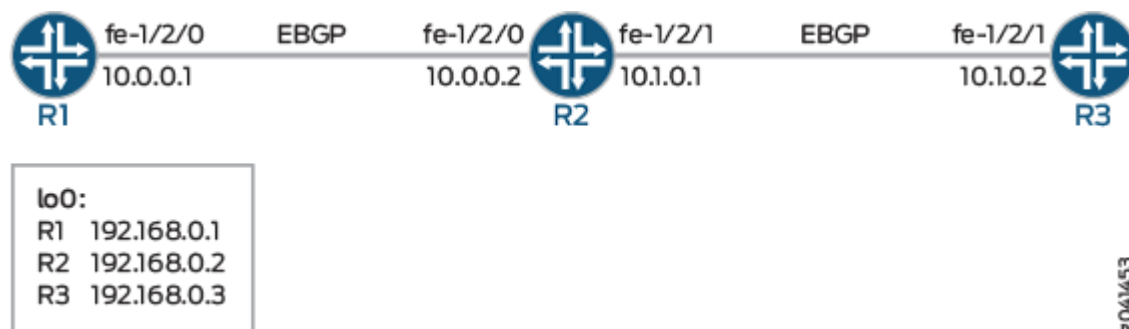
Figure 36: BGP Flap Damping Topology
