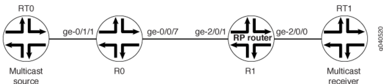
Figure 41: PIM Sparse Mode over an IPsec VPN
