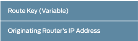
Figure 101: Leaf Autodiscovery Route Type MCAST-VPN NLRI Format
