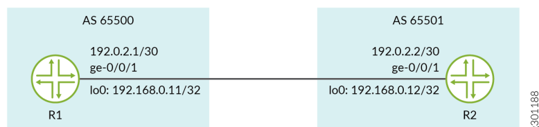
Figure 4: Topology for BGP Authentication
