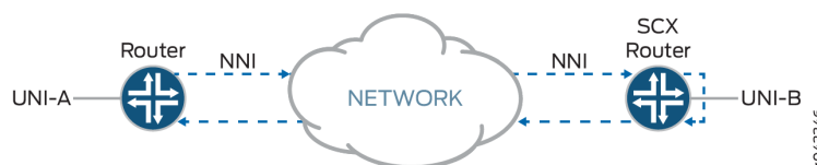
Figure 61: Testing End-to-End Service in Ethernet Loopback Mode
