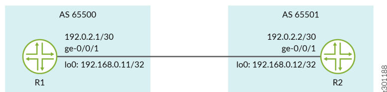
Figure 4: Topology for BGP Authentication
