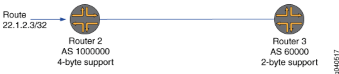
Figure 27: 4-Byte Capable Router Having a Peer Relationship with a 2-Byte Capable Router Using a 4-Byte AS Number
