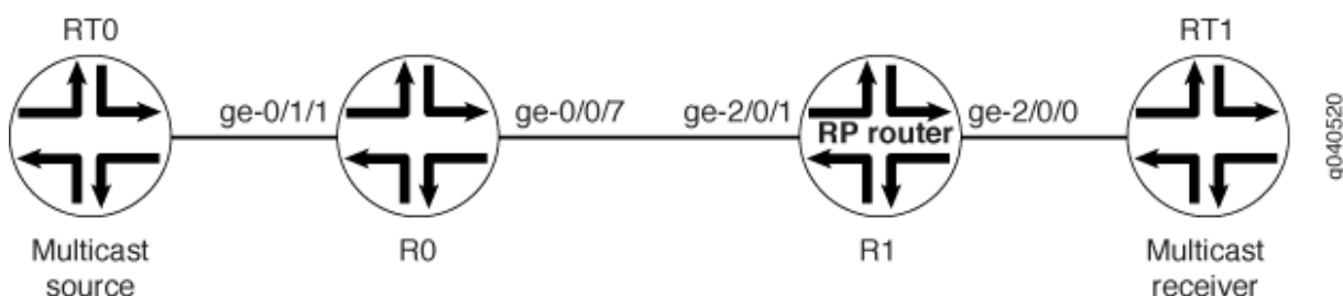
Figure 41: PIM Sparse Mode over an IPsec VPN
