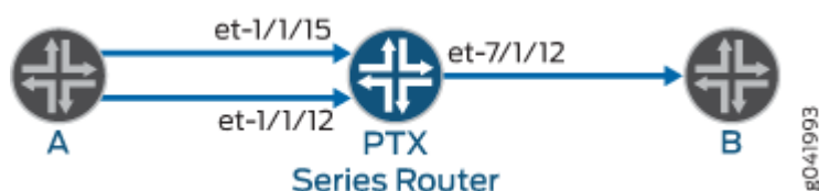
Figure 59: Topology for Configuring Strict-Priority Scheduling on a PTX Series Router
