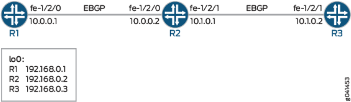
Figure 90: BGP Flap Damping Topology
