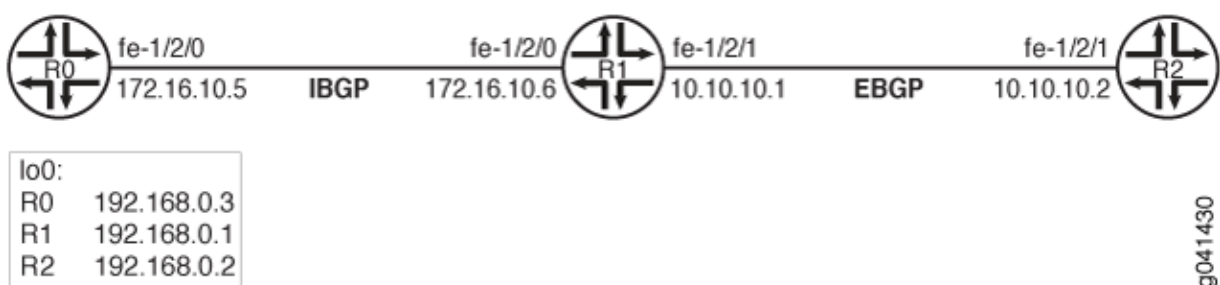
Figure 93: BGP Error Handling Example Topology
