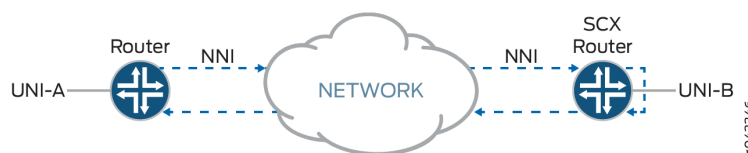
Figure 51: Testing End-to-End Service in Ethernet Loopback Mode
