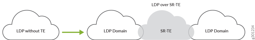
Figure 4: Interconnect LDP Domains over SR-TE in the Core Network
