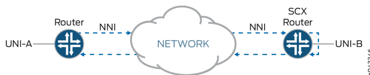
Figure 57: Testing End-to-End Service in Ethernet Loopback Mode
