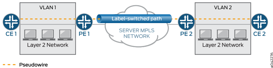
Figure 105: Traditional Layer 2 Point-to-Point Services
