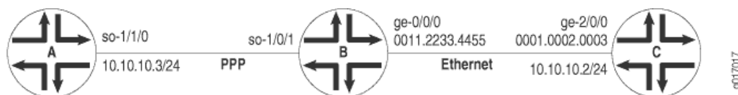
Figure 105: Sample Topology of Layer 2.5 Translational Cross-Connect
