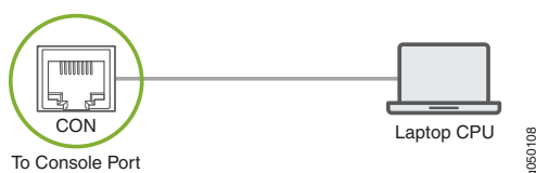
Figure 63: Connecting the QFX Series Directly to a Management Console
