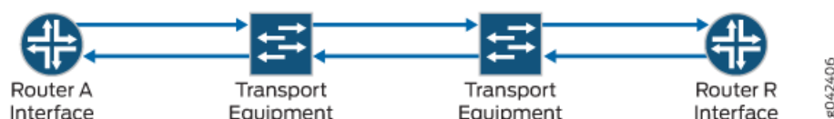
Figure 6: Two Router Interfaces Connected Through Transport Equipment
