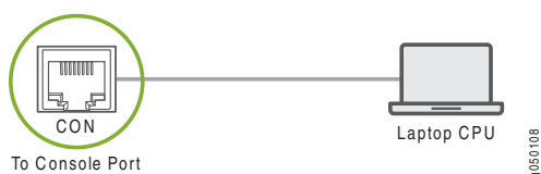
Figure 41: Connecting the QFX Series Directly to a Management Console
