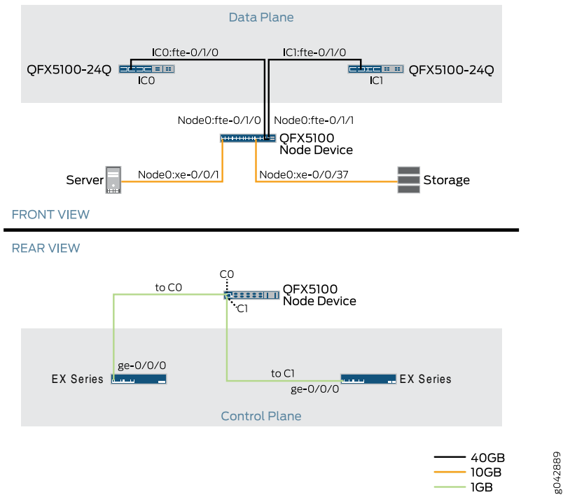
Figure 90: QFX5100 Node Device Data Plane Connections to an QFX5100-24Q Interconnect Device for QFX3000-M QFabric System
