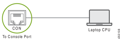
Figure 31: Connecting the QFX Series Directly to a Management Console
