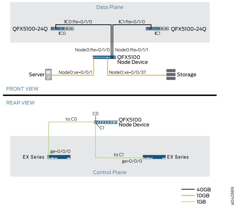
Figure 11: QFX5100 Data Plane and Control Plane Connections
