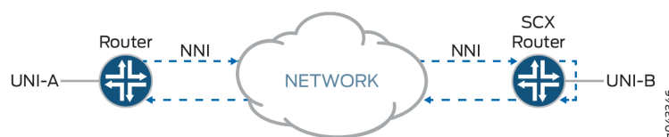
Figure 57: Testing End-to-End Service in Ethernet Loopback Mode
