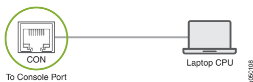
Figure 23: Connecting the QFX Series Directly to a Management Console
