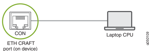
Figure 63: Connecting the QFX Series Directly to a Management Console
