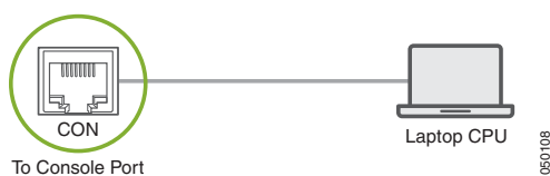
Figure 73: Connecting the QFX Series to a Management Console Through a Console Server
